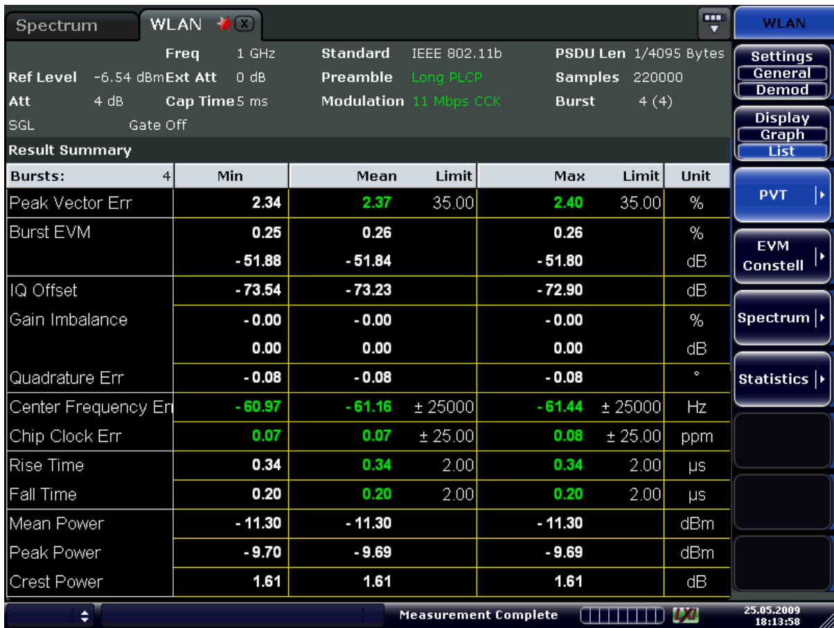
Fig. 3-12: Result summary list for measurements on DSSS/CCK/PBCC signals
